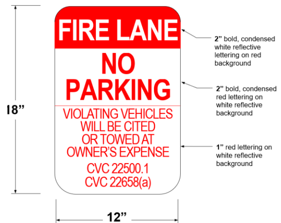
Figure 5 – Fire Lane No Parking Signs
