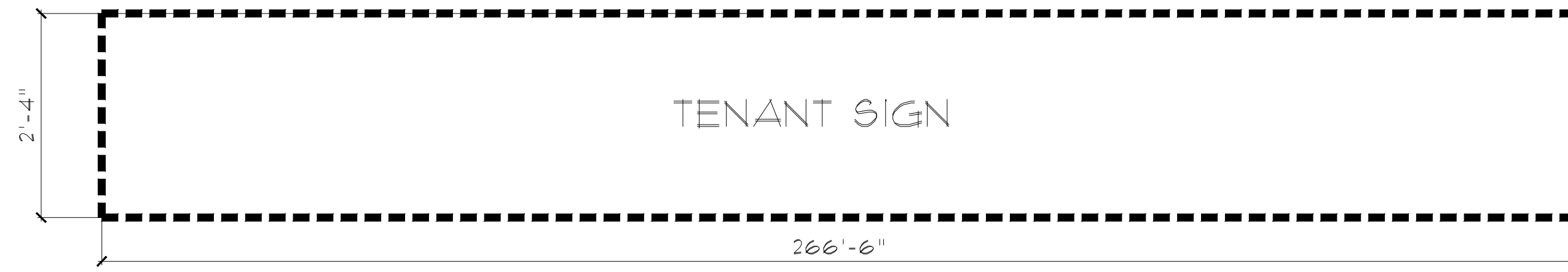
WALL MOUNTED INTERNALLY ILLUMINATED LED SIGN
