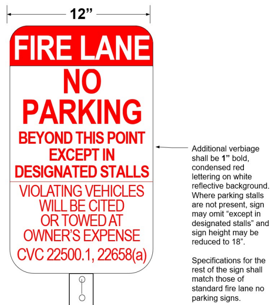
Figure 9 – Specifications for Alternative Fire Lane No Parking Signs
