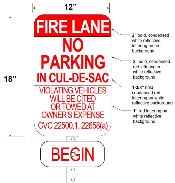
Figure 12 – Specifications for Cul-de-Sac Fire Lane No Parking Signs
